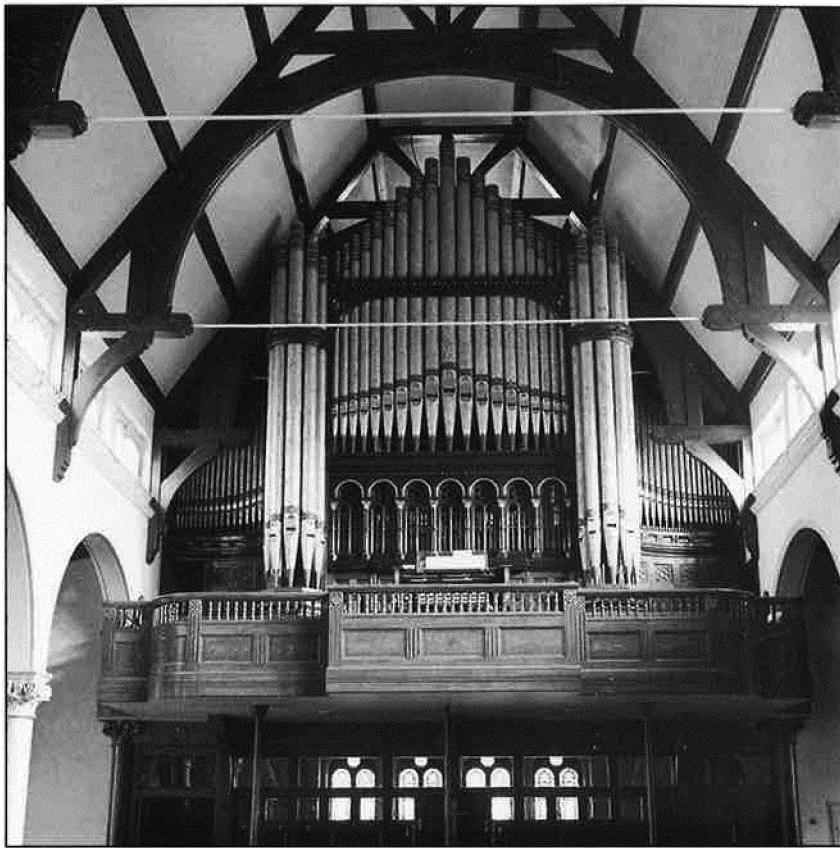
In 1883, Hilborne Roosevelt incorporated electropneumatic action for the Echo division in his 75-rank opus 113 built for First Congregational Church, Great Barrington, Massachusetts. Three other manual divisions used tubular-pneumatic action. The organ is built on ventil wind-chests and exists intact except for replacement of the console and the tubular action with electric primaries ca. 1935. BELOW: The console of this organ photographed in 1928 shows the switches of a player-settable combination action behind glass doors flanking the music rack.
