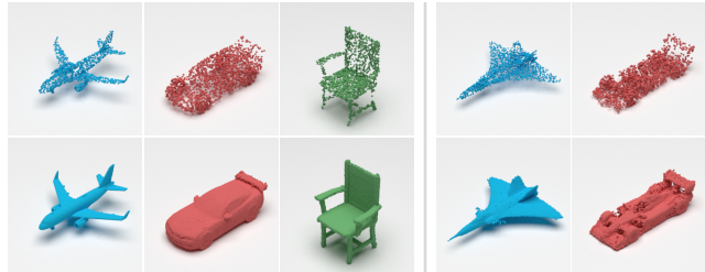
Figure 6: Point cloud upsampling examples. Top: original point clouds with 2048 points. Bottom: we upsample them by 50x to 102k points. Left: Our inpainting technique yields high-quality point clouds. Right: Artifacts may appear occasionally, especially on complex, irregular structures. Note: figure is rendered with a smaller point size.
