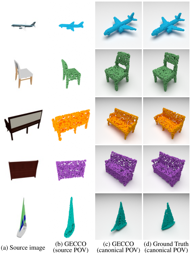
Figure 2: Image-conditioned generation. We condition denoising diffusion models with images (a) in a geometrically-principled manner. Our model can reconstruct the shapes accurately from that view (b), and also generate plausible completions for regions not visible in the image (c, d), even under drastic occlusions (rows 3-5).
