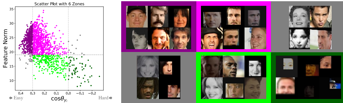
Figure 5. Actual training data examples corresponding to 6 zones. A pretrained AdaFace model is used as a feature extractor.
