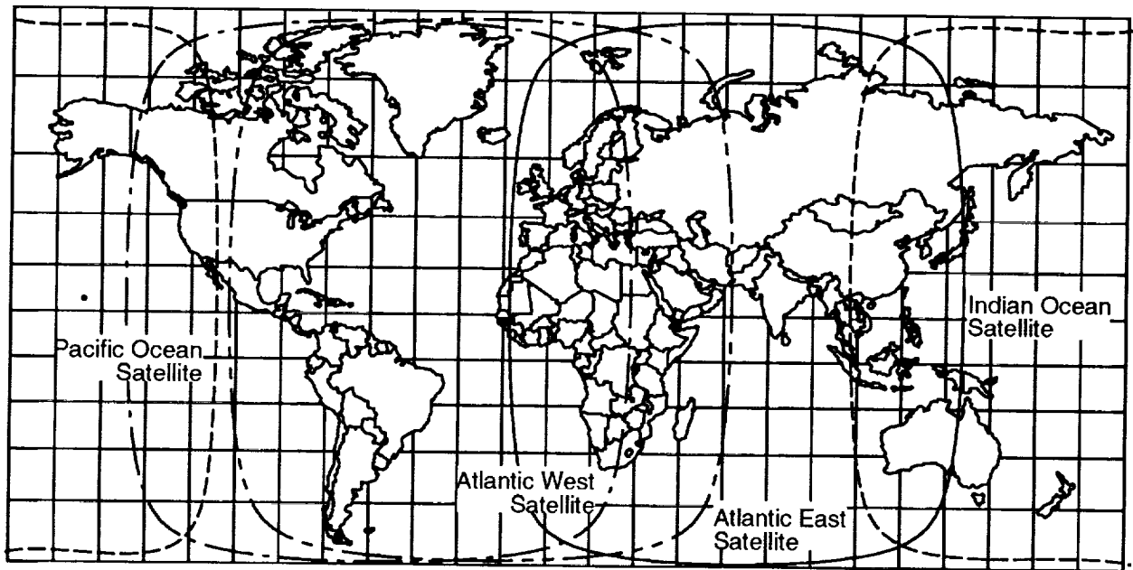
Figure 2. Global INMARSAT Satellite System Coverage
