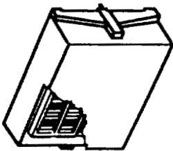
TRANSPORTER ENERGY STORAGE SUBSYSTEM
