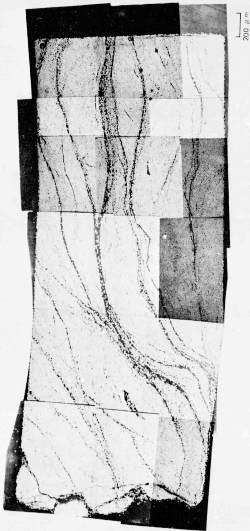
Figure 22. Tape Map of Cross Section of HMS Graphite Fiber Reinforced 7740 Glass Matrix (GC 281) Hot Pressed at 1473 K, Slurry B
