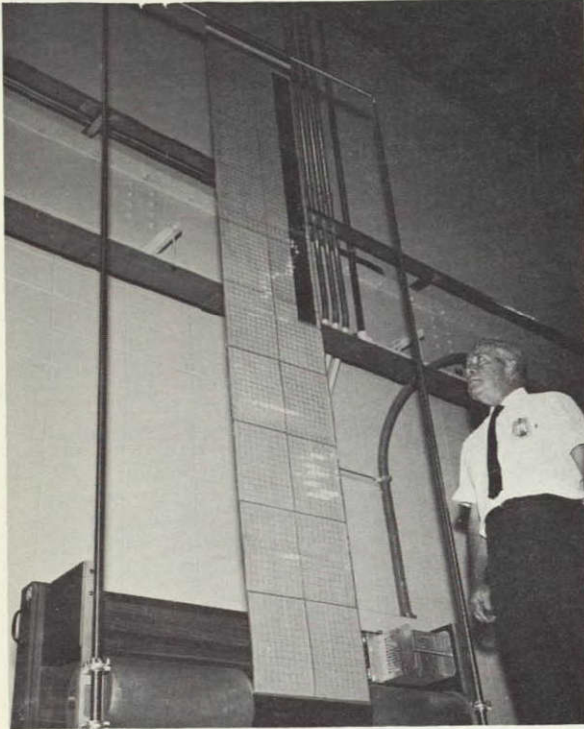
Figure 4.7-10. Engineering Model of Rollup Solar Array
