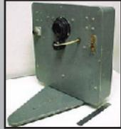
Because the rapatronic camera could only take one photo, banks of cameras were needed to photograph a single nuclear test.
