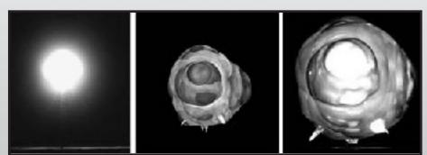
Rapatronic images captured in succession during an atmospheric tower test in the Snapper
