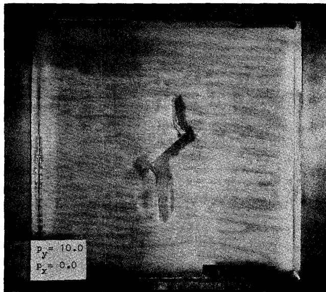
Fig. 10 Results of test on PMMA plate. Primary cracking only; no rupture occurs. From Ref. 23.
