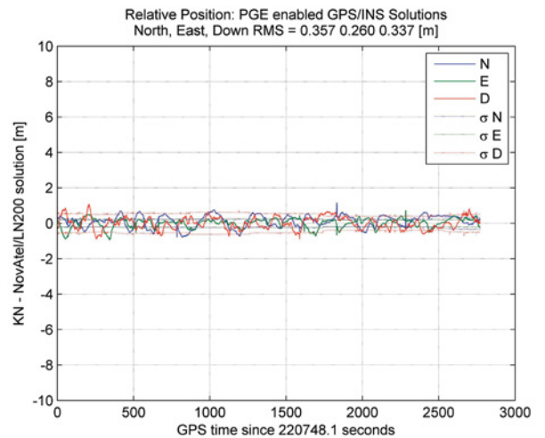
▲ FIGURE 10 Flight 1: Relative position of KN and NovAtel/LN200 PGE enabled GPS/INS solutions.
