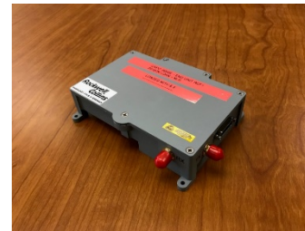
Small form factor, low size, weight and power for smaller aircraft at lower altitudes in higher-density environment. Improved waveforms, C-band frequencies, no ITAR restrictions
