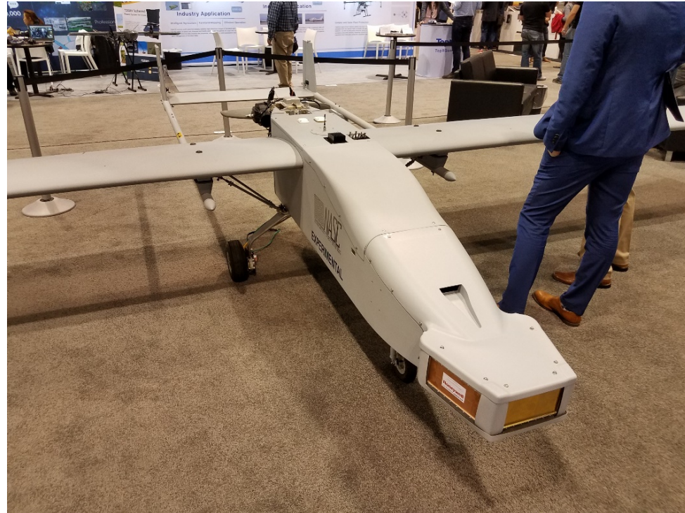
Tiger Shark with Honeywell RADAR Panels
