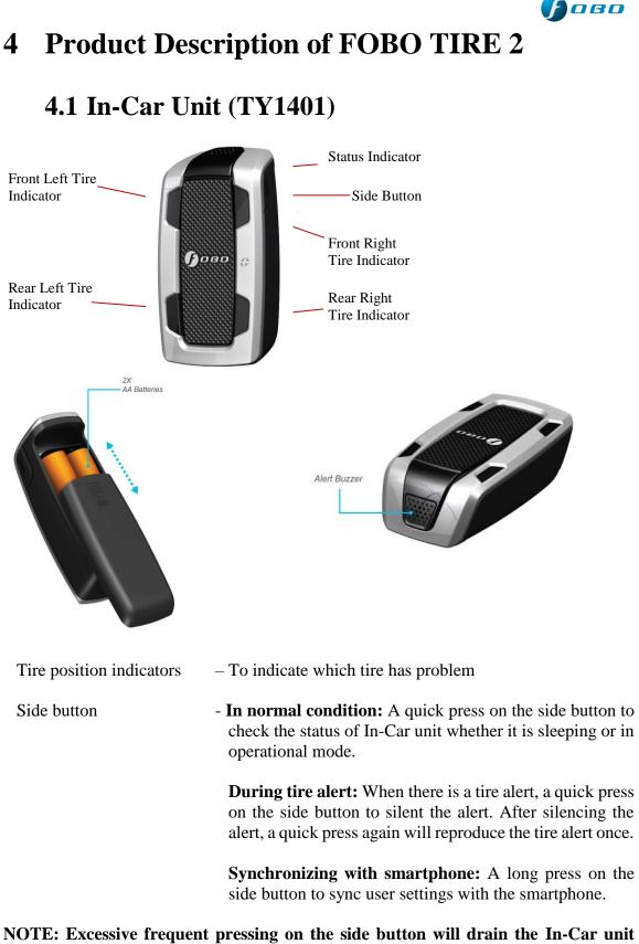
NOTE: Excessive frequent pressing on the side button will drain the In-Car unit battery.
