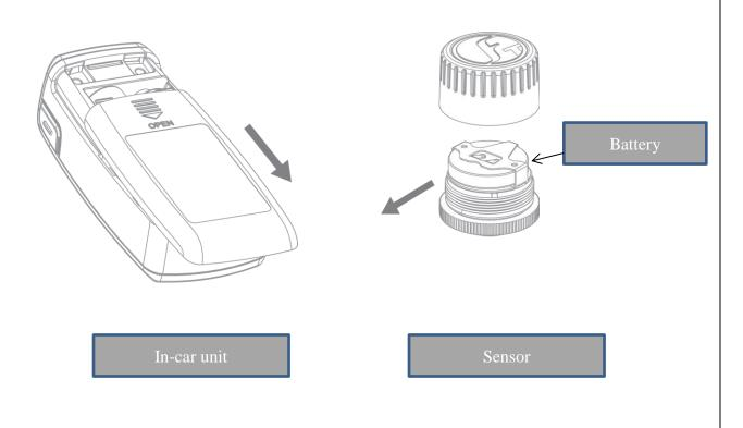
**Note:** It is recommended to remove sensor/in-car unit batteries if you are not going to use it for long time.
