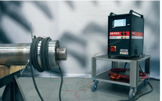
+ Crank shaft with inner ring and flexible inductor
