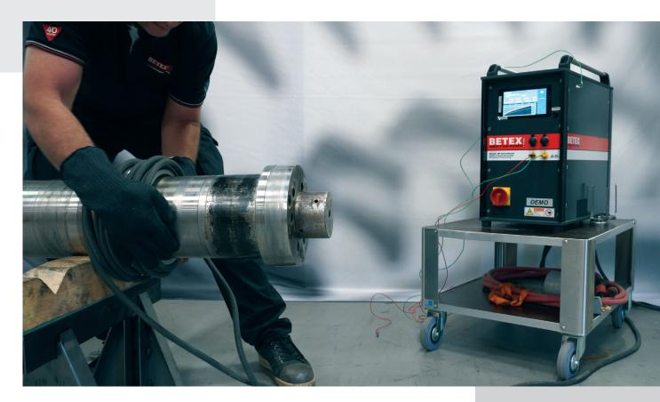
+ Crank shaft with inner ring dismantled in 1 minute
