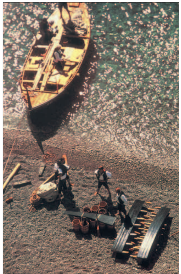
The "gaeta" turns from sailboat to finishing boat upon removal of the upper sideboard, beach of Palagruza (Croatia). The gaeta has a unique naval architecture combining two boats in one
