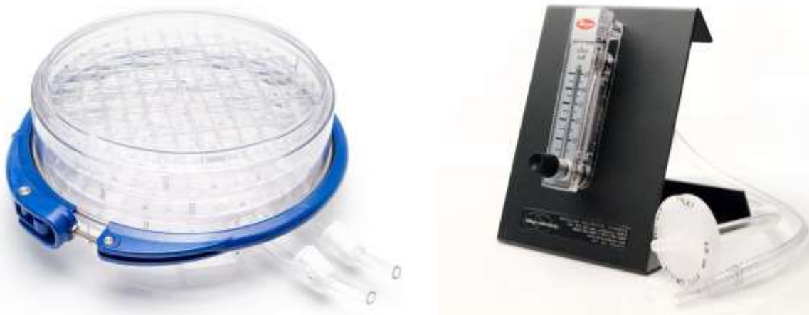
Figure 3.2: Modular hypoxia chamber used for hypoxic incubation. The chamber (left) containing cell culture plates was flooded with a gas mixture containing 1% \text{O}_2 , 5% \text{CO}_2 and 94% \text{N}_2 using the flow meter (right). Images from stemcelltechnologies.co
