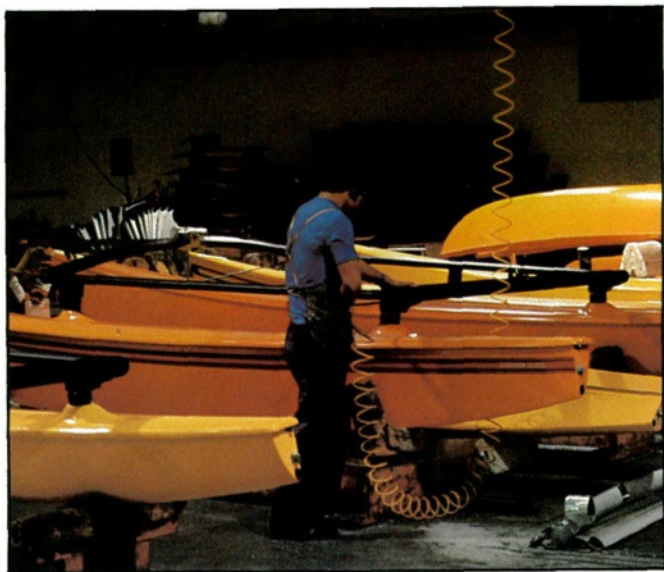
Each boat is completely assembled at the plant. Cross-bars are drilled to fit, and the hardware is mounted.
