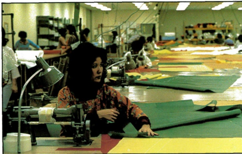
Hundreds of yards of colorful cloth pass through the sail loft at Hobie Cat each day. Cutters, hemmers, and seamers transform cloth into shapely sails.
