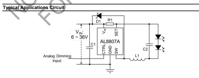
HIGH EFFICIENCY LOW EMI WIDE ANALOG DIMMING RANGE 36V 1A/1.3A BUCK LED DRIVER
