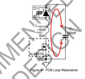
An example of good layout is shown in Figure 42 - the stray track inductance should be less than 5nH.
