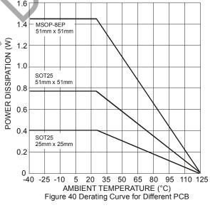
$P_{D(MAX)} = (+125^{\circ}C - +25^{\circ}C) / (250^{\circ}C/W) = 0.4W$  for single-layer 25mm x25mm PCB  $P_{D(MAX)} = (+125^{\circ}C - +25^{\circ}C) / (130^{\circ}C/W) = 0.77W$  for dual layer 51mm x 51mm PCB
