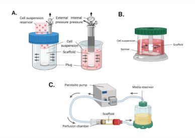
**Figure 6.** Dynamic seeding methods. **(A)** Vacuum seeding: using internal or external pressure forces to drive cells into scaffolds. **(B)** Centrifugal/rotational seeding: using rotational force to drives cells into the scaffold. **(C)** Perfusion seeding: mimicking the in vivo physiological conditions and biomechanical stress of blood vessels to aid cell attachment to the scaffold. (Created with Bio-Render.com [Accessed 30 January 2022]).
