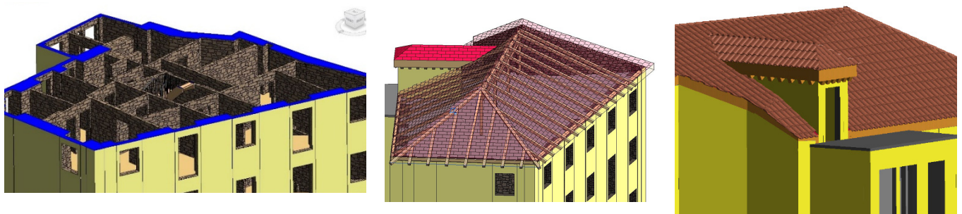
Figure 6. Model of the interior walls and roof.
