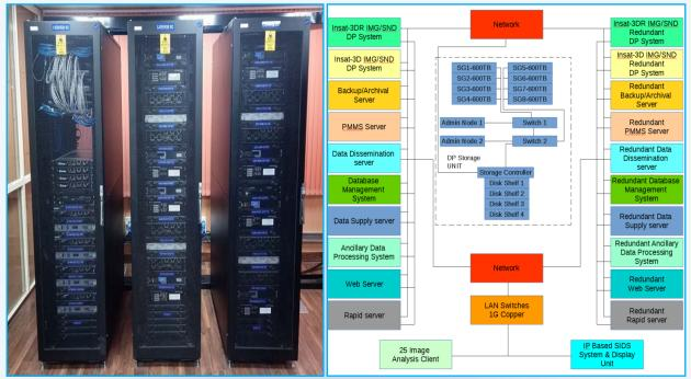
Fig. 43. Block diagram of MMDRPS system
