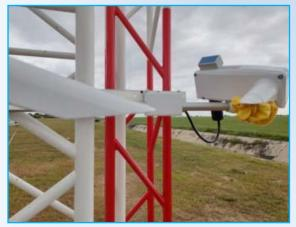
Fig. 15. Installation of Present Weather and visibility sensor at RGI airport, Hyderabad
