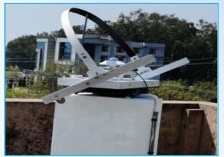
Fig. 7. Pyranometer for measurement of diffuse radiation
