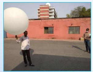
Fig. 4. Testing of GPS based Pilot-sonde manufactured in IMD Workshop New Delhi
