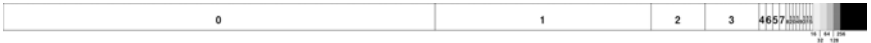
Figure 14.2. codes on the unit interval; \bar{0} = 0 , \bar{1} = 10 , \bar{2} = 110 , \bar{3} = 1110 , \bar{4} = 1110\ 0\ 00 , \bar{5} = 1110\ 0\ 10 , \bar{6} = 1110\ 0\ 01 , \bar{7} = 1110\ 0\ 11 , \bar{8} = 1110\ 1\ 000 , etc..
