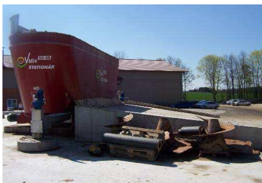
Fig.4. Feed-in container system for dry feedstock - maize silage and solid poultry manure [1]
