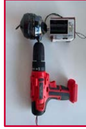
PICTURE 2: REELING SUBSYSTEM: CONSISTS OF AN ARDUINO MEGA THAT CONTROLS A SOLENOID REEL PRESSED BY A SOLENOID
