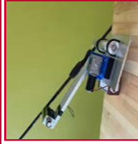
PICTURE 1: CASTING SUBSYSTEM: CONSISTS OF A GEARED MOTOR TO PRIME THE FISHING ROD ON A TORSION SPRING, RELEASED BY A SOLENOID
