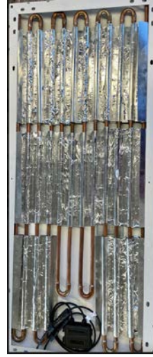
Fig. 1: Copper heat exchanger inside PV panel
