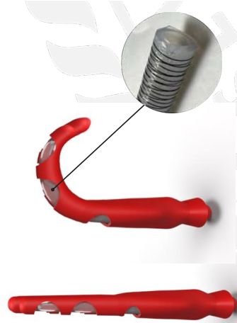
Figure 3: Finger Design with Actuation
