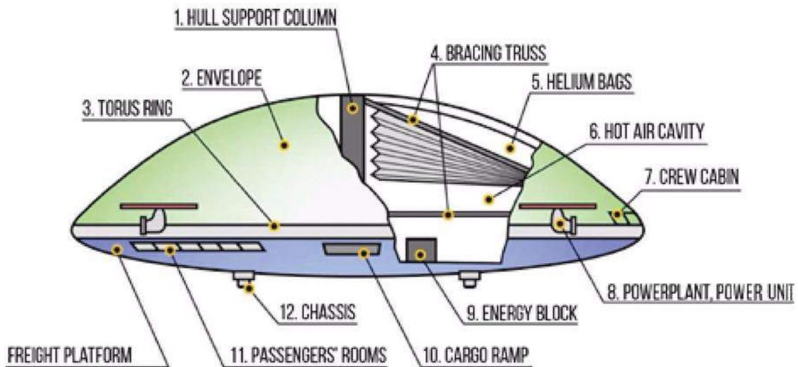
*General arrangement of an Aerosmena aeroplatform. The rigid hull structure includes the central hull support column, the torus ring around the periphery & the internal bracing trusses. Source: AIDBA*
