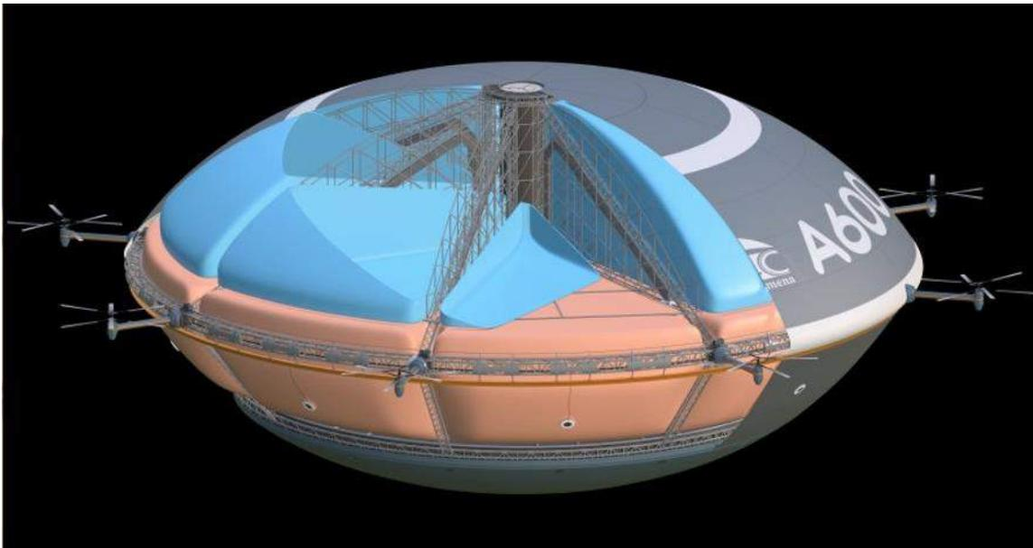
*A600 cut-away drawing showing the primary internal structures: the central support column, the radial bracing trusses, and the circumferential torus ring, which supports the propulsion units. The lifting gas cells (blue) and the hot air cells (ochre / reddish color) are installed in the sectors between the bracing trusses.*
