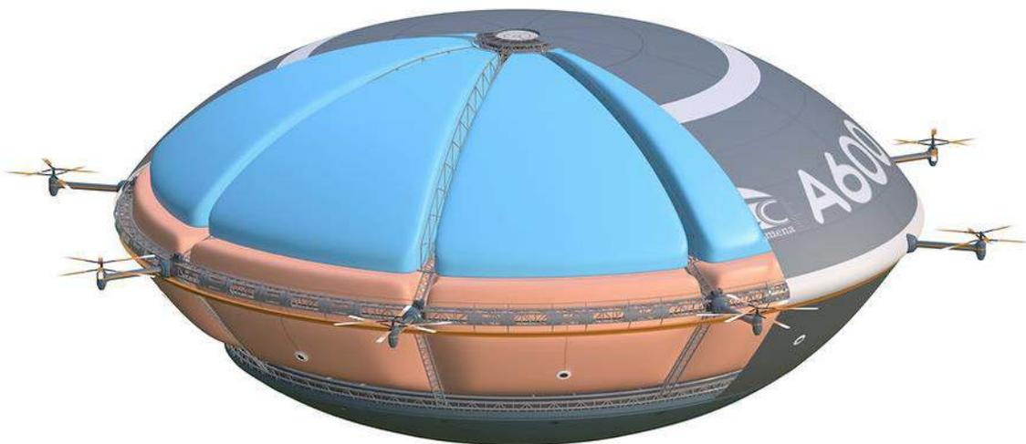
*A600 with the outer shell pulled back to show the placement of lifting gas cells (blue) and the hot air cells (ochre / reddish color).*
