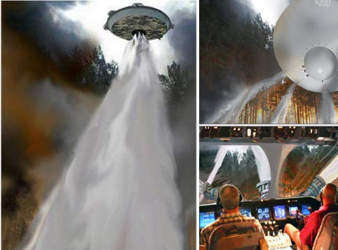
*Renderings of an A200 fighting a forest fire with a bulk water drop (left) and directional water cannons (right). Source: AIDBA*
