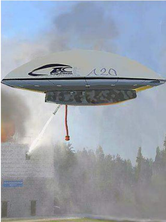
The 20-metric ton (22-ton) payload A20 will be the prototype for the entire Aerosmena family. This 70-meter (230 ft) diameter utility aeroplatform can be configured for a variety of missions, such as:
