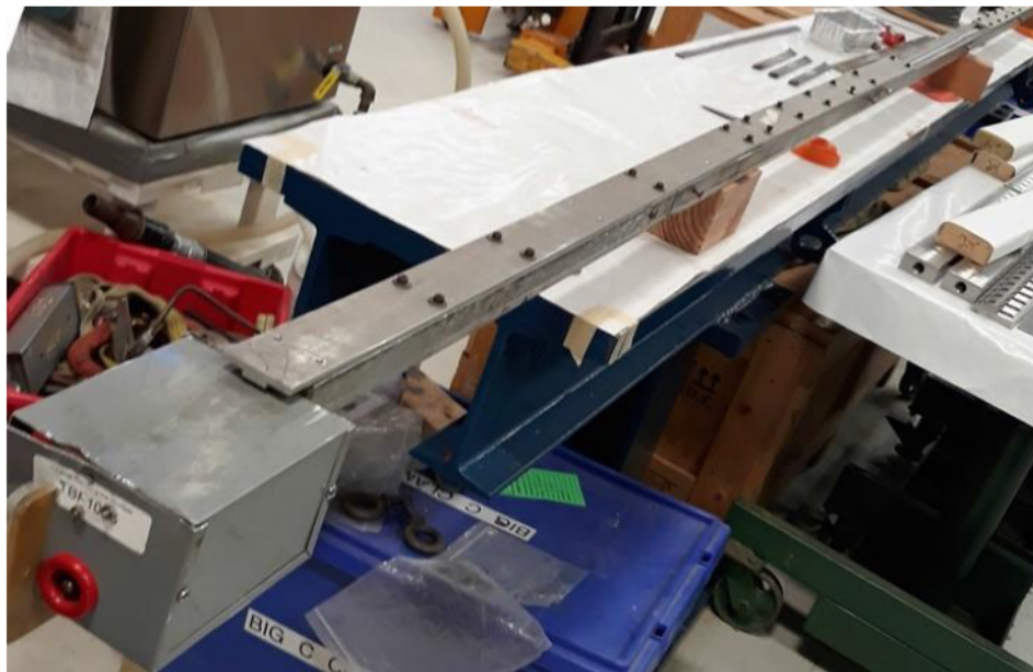
Figure 41: Bus Soldering Fixture for Q1/Q3 and Q2 busses (located in ICBA).
