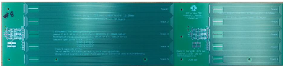
Figure 96: 220 mm and 110 mm long multi-layer PCB probes.
