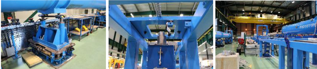
Figure 64: Existing LHC dipole magnet installation tooling.
