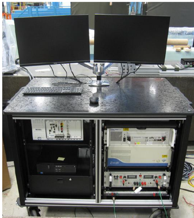
Figure 98: Fermilab SSW DAQ system.
