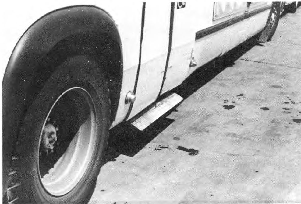
FIGURE 3.3-3: DRIFTING SAFETY BARRIER ON GMC LIFT
