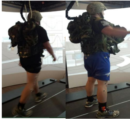
Figure 1. Subject Load Carriage Simulation on GRAIL system
