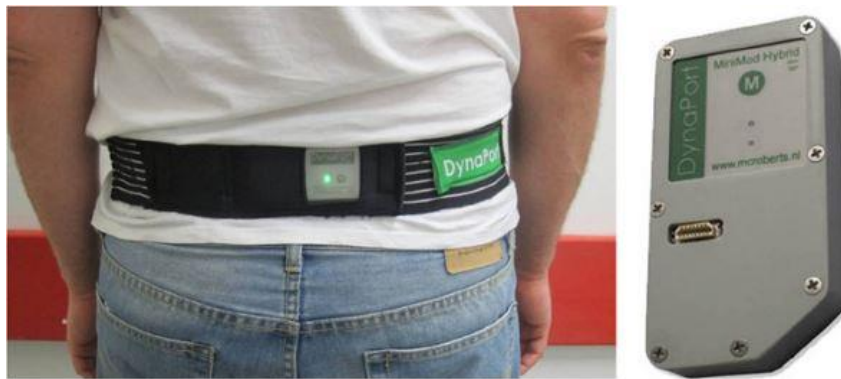
Figure 2-7. Utilizing Inertial Measurement Unit to assess the Activities of Daily Living of Subjects (Weiss et al., 2013)
