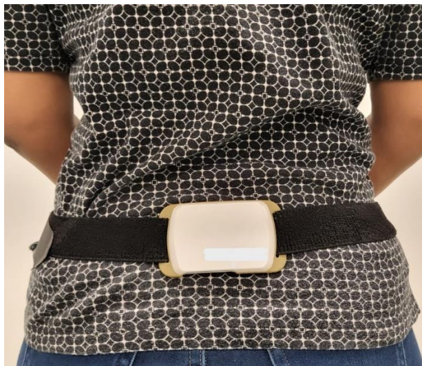
Figure 3. DynaPort MM+ IMU device is affixed on the participant's sacrum region to perform 3 days of Activities of Daily Living data collection
