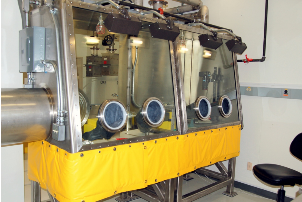
Figure 1. CCL glovebox used to visually inspect graphite samples, perform initial dimensional measurement, and repackage samples for storage in the irradiated graphite vault located in Lab C-19
