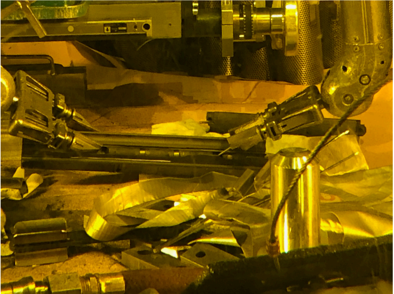
Figure 12. 240-degree sector of graphite body with exposed center section. Shiny samples are can design used for HOPG.
