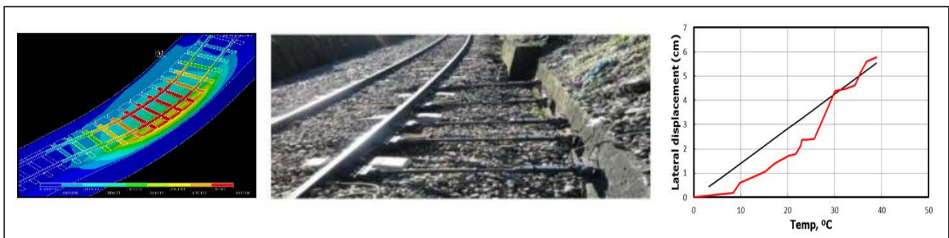
Fig. 4: 3D FEM lateral displacement results (left), real test (mid) and results comparison for \Delta T and validation (right).
