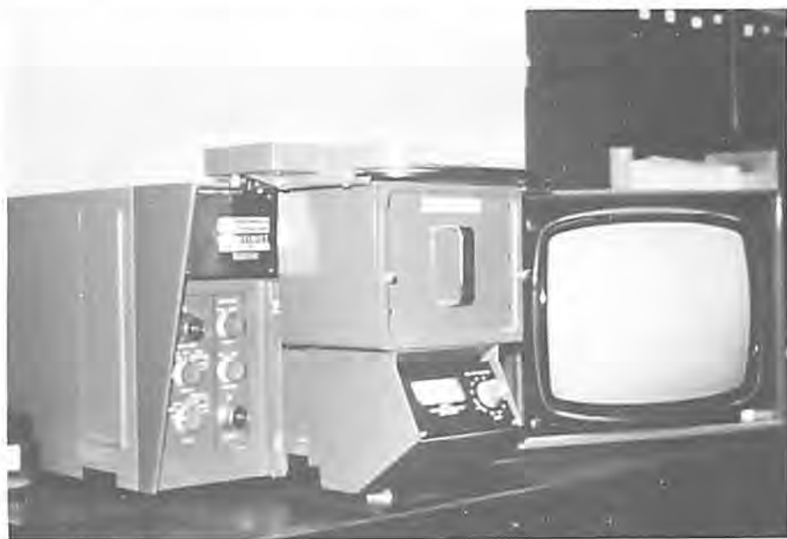
Fig. 2 - Image analyzing system at the Illinois State Geological Survey. To the far left is the processing and control unit. The meter, where areas and counts are read, is located in the lower center. The monitor is to the right. The source material is placed on the platform in the upper center.
