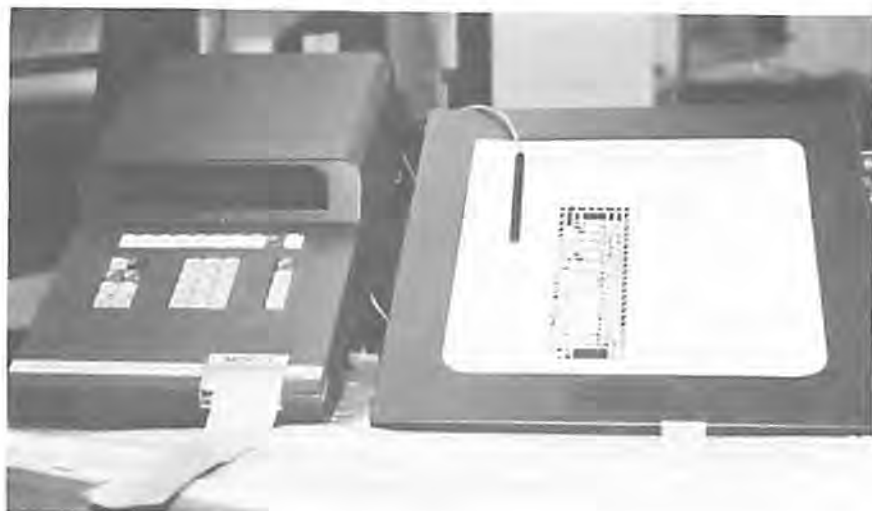
Fig. 11 – Image analyzing system at Northeastern Illinois University. This system is not a video-type system. It reads areas and determines counts using a pen and magnetic board. This system, made by Carl Zeiss, features a digital display and paper tape printer.
