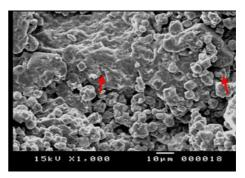
Fig. 20. The presence of granules that are not coated with Klucel G
