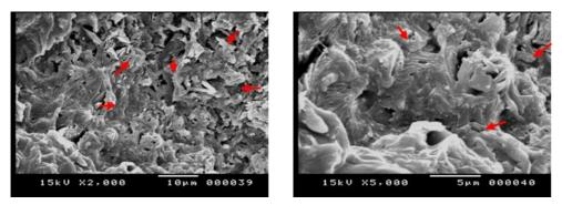
Fig. 27. The formation and flowering of sodium sulfate salts directly above the granules, having the film coated with Klucel G
