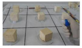
Fig. 2. The application of the consolidation materials using spray
