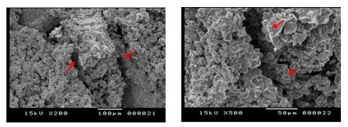
Fig. 24. The cracks are not filled with the Paraloid B72
