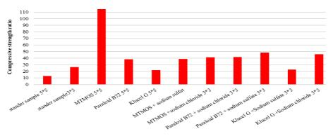
Fig. 13. The results of the pressure test for stone samples after the strengthening process
