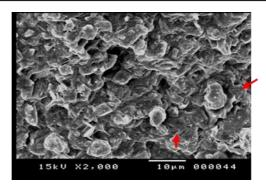
Fig. 28. The crystals of sodium chloride salts inside the pores of Klucel G
