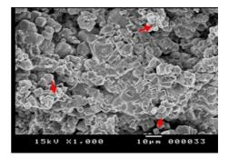
Fig. 26. The formation and flowering of sodium chloride salts on the membrane of the booster material MTMOS coated for the sample granules
