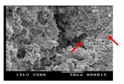
Fig. 18. The cracks are full of the MTMOS consolidation material
