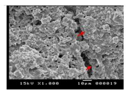
Fig. 21. Cracks not filled with Klucel G
