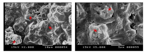
Fig. 30. The formation and flowering of sodium chloride salts inside the pores and granules of stone reinforced with Paraloid B72
