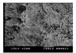
Fig. 22. The spread of Paraloid B72 inside the limestone pores
