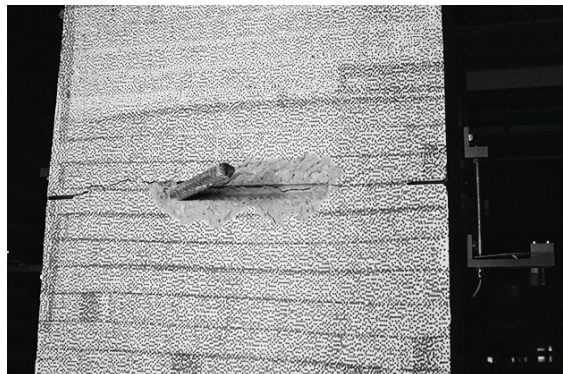
Figure 3.8: Picture after failure of specimen PM31 with spalling failure of the concrete cover.
