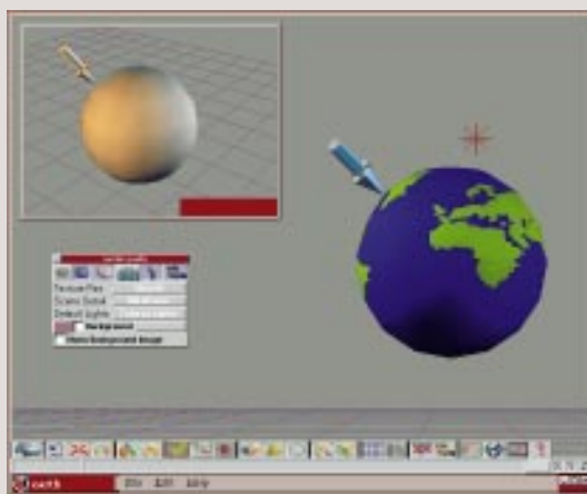
The Fountain interface, with a VRML scene of the globe in the main window, and a panel showing a separate, non-textured version of the same scene from a different angle. The spear-shaped object pointing at the globes is a pointer put there by Fountain to show that the globe is the currently selected object
