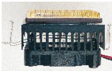
The 6x86 incorporates Pentium Pro-like architecture that fits into a 296-pin P54C socket
