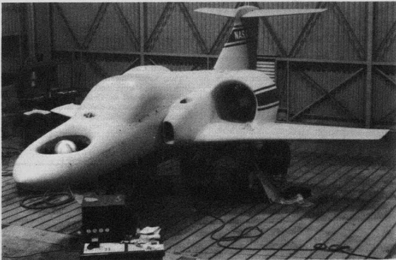
A 0.7 scale model of a conceptual VTOL (vertical take-off and landing) aircraft being studied as part of a NASA-U.S. Navy lift cruise fan research and technology aircraft program. The model is being readied for testing in the Ames 40 by 80 Foot Wind Tunnel. Such an aircraft would use fans driven by two jet engines for direct lift and forward propulsion.
