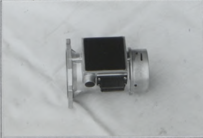
H) Injection system (Air flow meter)
