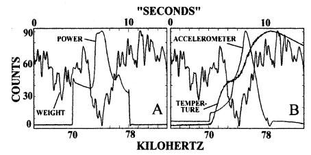
Figure 4: The weight fluctuation in the device shown in Figures 1 and 2 was swept with a sinusoidal signal. The weight is recorded in  $\Delta DC$  counts, 66 counts scaling to 0.1 gram. The power trace shown in panel A peaks at 105 Watts. The corresponding thermistor (temperature) and accelerometer traces shown in panel B were not absolutely calibrated.
