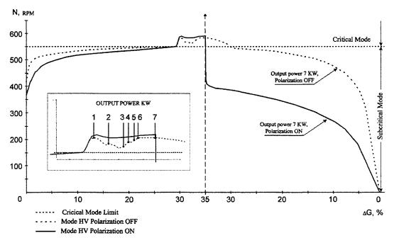
Fig.4. A diagram illustrating various operation regimes of the converter, -G, +G changes in weight of the platform vs. rpm
