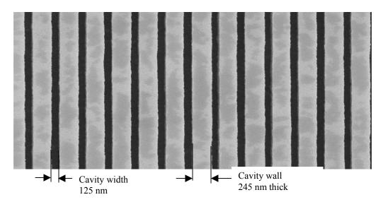
**Figure 5**. SEM photograph of portion of the gold cavity array. Each cavity is actually100 um long. The entire array is 100 um wide (magnification 37,000; 15kV).
