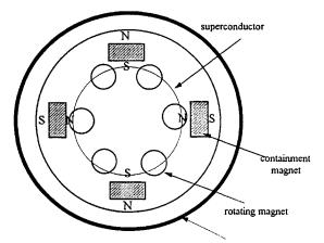
position of 13.56MHz coil Fig. 9: Positioning of containment magnets to prevent the superconductor rotating uncontrollably
