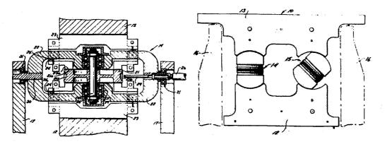
Figure 6 Setup of Rotating Test Mass (2 Axis) and Generator (Left) and Detector (Right) Position<sup>15</sup>
