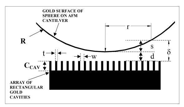
**Figure 6.** Distance definitions, illustrating actual cavity depth ( $C_{CAV}$ ), individual cavity width (w), cavity wall thickness (t), separation distance (*d*), local sag (*s*), and local separation distance ( $\delta$ ).
