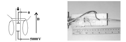
Figure 2. Diagram and photo of NMR coil and flow arrangement for E-field experiment
