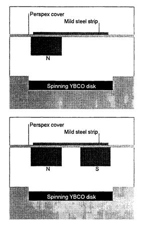
Fig. 6: Sample magnet configurations
