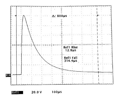
Figure 3. Typical pulse shape at maximum capability: 2400 A peak into a 0.05  $\Omega$  resistive load. When driving the thruster antenna through our coaxial cable, the pulse height was reduced to about 1200 A, at rise and fall times of about 20  $\mu$  s and 400  $\mu$  s, respectively.
