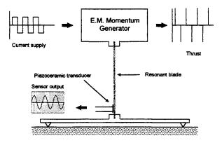
Fig. 6 Micromotion sensing concept.
