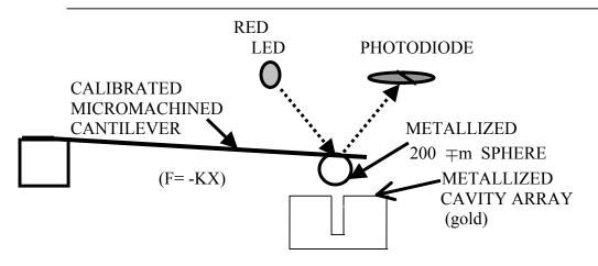
**Figure 2.** Schematic of Atomic Force Microscope measurement of the vacuum force between a metallized sphere on a cantilever and a rectangular cavity etched in gold (not to scale).
