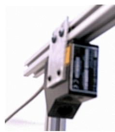
Fig. 4 Laser position measurement device.
