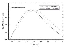
Fig. 2: Superluminal propagation for the tunneling pulse
