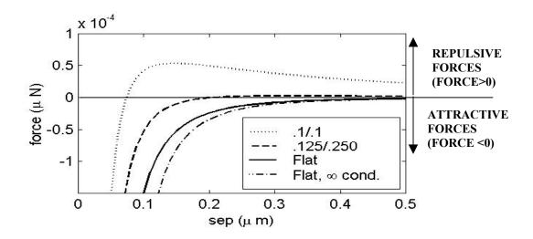
**Figure 7.** Force vs. distance d for a 100 um square cavity array with 1) the target dimensions, cavity width w = 0.1 um, wall thickness t=0.1 um, depth Ccav = 1.0 um deep; 2) the best fabricated cavity, width w=0.125 um, thickness 0.250, depth 0.5 um deep. The two uppermost curves show the force for the sphere above the cavity arrays. The solid curve shows the attractive force for a flat surface, with no cavities. Conductivity corrections are included. The sphere diameter is 210 um.
