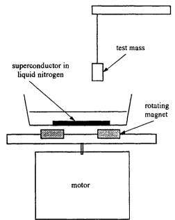
Fig. 7: Rotating field apparatus
