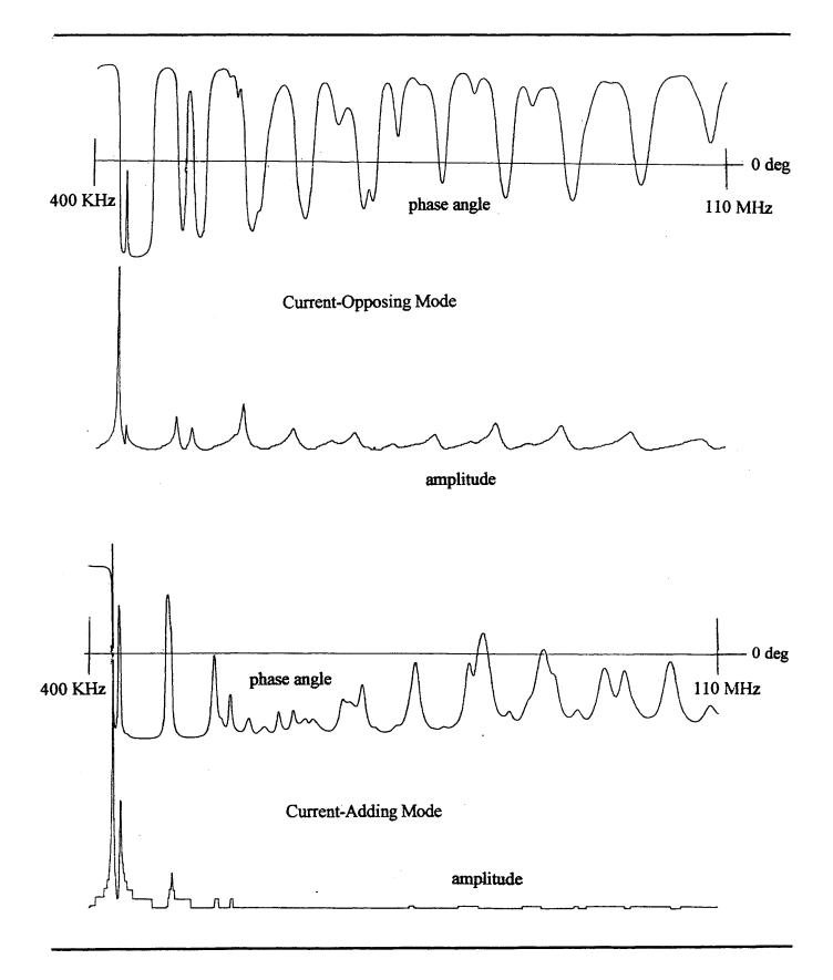
Fig. 10 - Resonances for "Tear-Drop" Toroid
