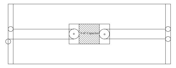
*Figure 2* Top view of "Mach Guitar" arrangement. The capacitor is suspended between pairs of tensioned wires that provide the restoring force for the mechanical oscillator. Capacitor drive voltage is supplied through the wires.
