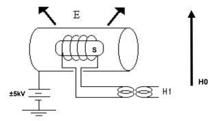
Figure 1. NMR "can" arrangement. External magnetic field, H0, is perpendicular to the radio frequency field, H1, applied through a coil wrapped around the proton sample, S. The 5kV electric field is applied outside the can leaving a constant 5kV potential inside.
