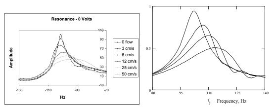
Figure 3. Measured NMR lines (left) and calculated (0,12,25,50 cm/s) for zero E-field and flows from 0 - 50 cm/s.
