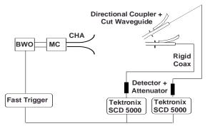
**Fig. 1:** Time-domain experimental setup
