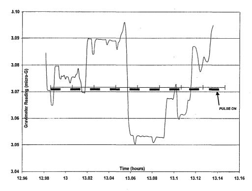
Figure 3 Gravimeter reading with 9 pulses of 1100 gauss, 45 Hz levitation field applied to 10 cm YBCO superconducting disk.
