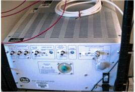
*Fig.* 5 Trek Model PO923A HV Power Amplifier, used for driving the capacitor at 2 kV and 400 mA.
