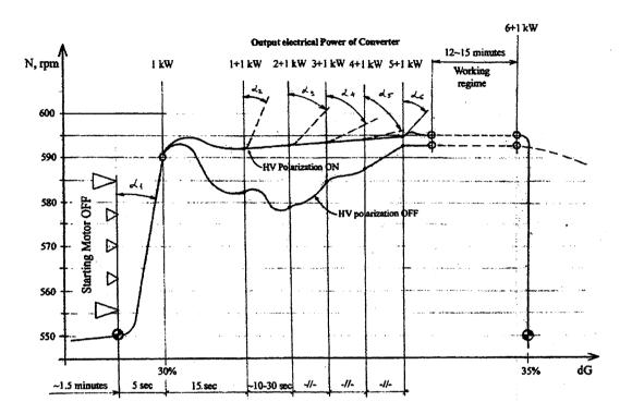
Fig.5 Diagrams of rotor accelerating and loading of the converter.
