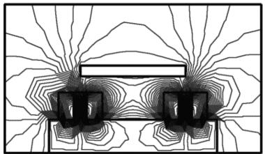
Magnetic Flux Lines around 1/2 of toroidal disk created by one solenoid assembly. Note the expulsion of flux from the superconductor.
