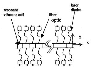
Figure 4: Laser Diodes and Linear Array
