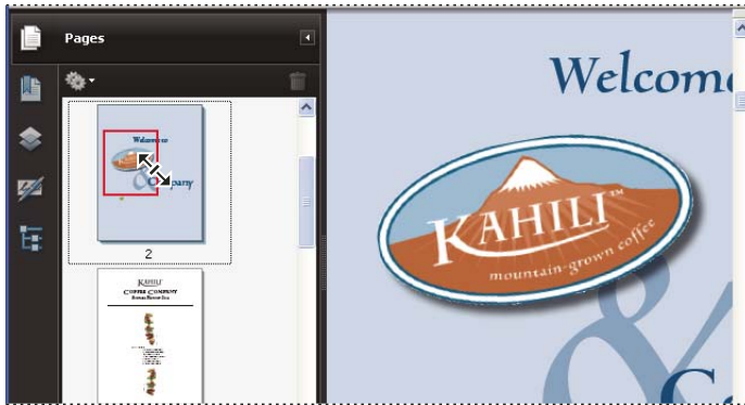
A page-view box in a page thumbnail indicates the area of the page currently showing in the document pane.
