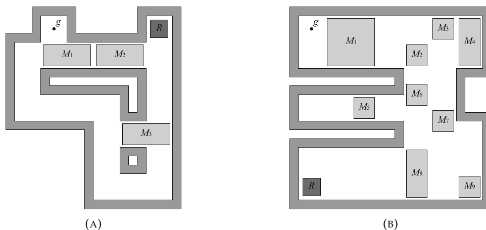
FIGURE II.10: NAMO problem examples solved by Van den Berg et al.’s algorithm [5]. (A) NLNM problem where the robot must pass by M_2 , then move it to the right, then move M_3 to the left, navigate through the bottom U-turn, move M_3 again but to the right, to finally move M_1 in the space left by moving M_2 . (B) Axis-aligned version of an L_kM problem initially solved by Stilman & Kuffner’s reverse-planning algorithm [46], where the smaller obstacles must be moved first to allow the necessary manipulation of M_1 .
