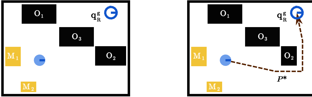
(A) The way to the goal is blocked by static obstacles (B) A plan avoiding all obstacles exists, but no better plan can be found by manipulating M_1 or M_2
