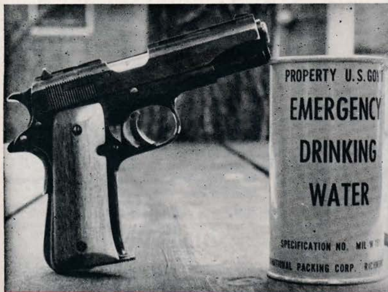
The Llama "Especial" .32 ACP is another good gun for non-serious shooting. This one has had a trigger shoe fitted to greatly improve pull.
