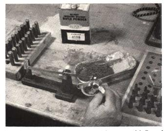
Weighing layout (hold to .01 grain) has capped hulls end up at left, powder scale and fixin's, charged cases right. C AN YOU GET bench rest accuracy from cast bullets? Consistent minute-of-angle groups from lead-alloy slugs? With careful handloading, both are entirely possible.
