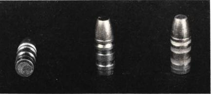
Bullets must be cast sharp, flat bases to take lube and gas checks (at right).
