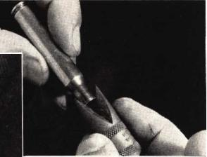
Trimming case neck leaves slight burr. Remove inside and outside by chamfering cutter. Herter tool has right bevel shape.
