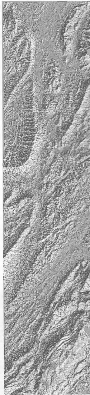
Figure 8: The shaded relief surfaces of the Tubau area. The shaded relief model depicts a pseudo-illumination of the land surface from 0° azimuth and 30° elevation.
