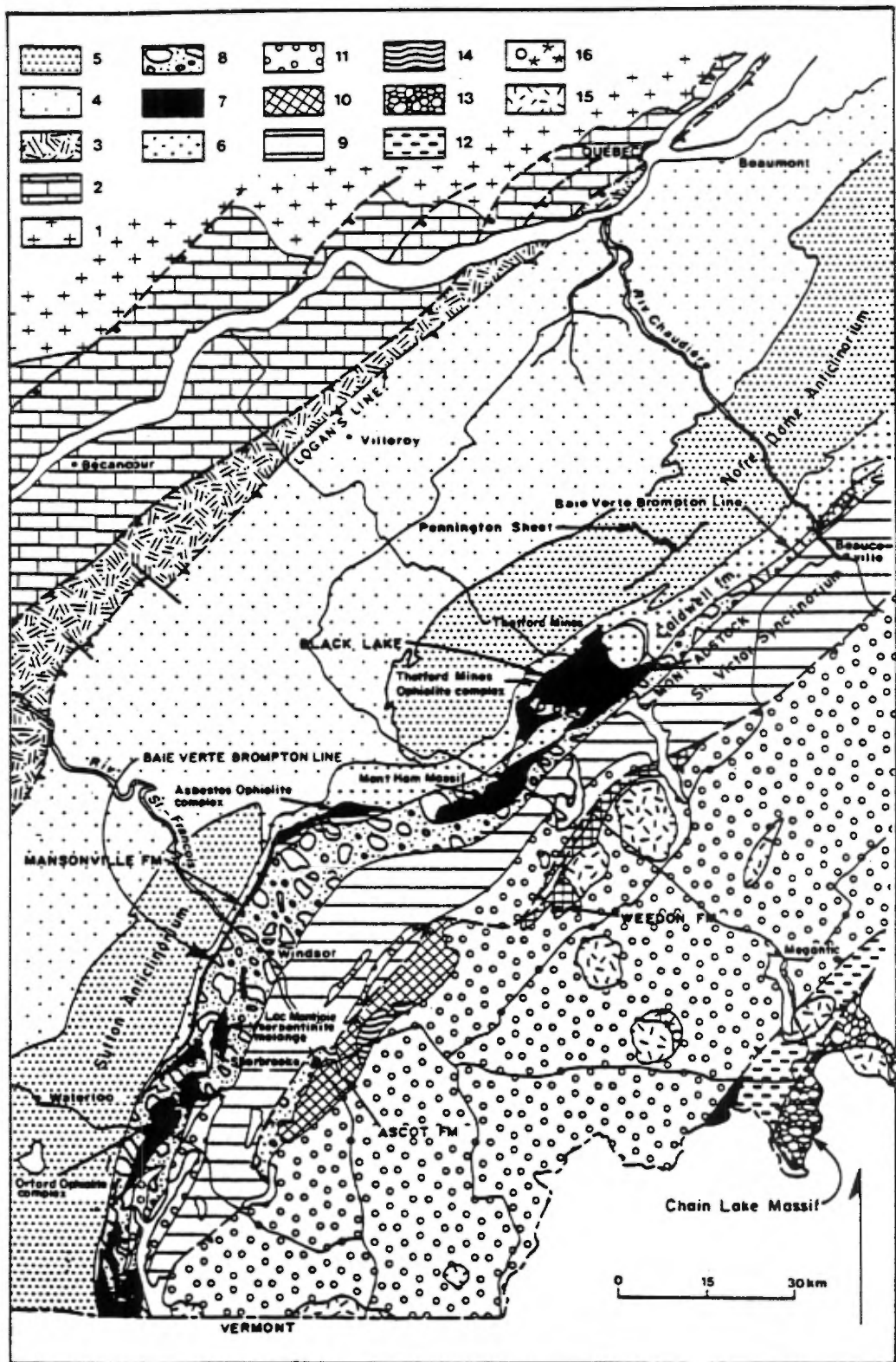
Figure 2. The Baie Verte-Brompton Line and major rock units of the Quebec Eastern Townships: 1) Grenville basement (Pe); 2) St. Lawrence platform ( \epsilon-0 ); 3) Foreland thrust belt (0); 4) Allochthones of the external domain ( \epsilon-0 ); 5) Allochthones of the internal domain (mainly Sutton-Bennett schists) ( \epsilon-0 ); 6) Caldwell Gr. and Mansonville Fm. ( \epsilon ); 7) ophiolites ( \epsilon ); 8) St. Daniel and Brompton Fms. (Mélange) (L.0); 9) St. Victor synclinorium (Magog Gr.) (M.0); 10) Ascot-Weedon Fms (L 0-M.0); 11) Connecticut Valley-Gaspé synclinorium (S-D); 12) Frontenac Fm. (0?); 13) Chain Lakes Massif (Helikian); 14) Ordovician granites; 15) Devonian granites; 16) Mesozoic alkaline intrusive rocks.
