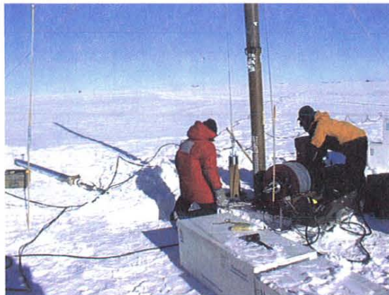
Fig. 5.42. Bladder being sent down into one of the two holes at South Pole for subsequent sampling of firn air. The 10-m-long bladder was pressurized to inhibit airflow from above while firn air was sampled through a 15-cm-high, stainless-steel-lined open chamber situated between the bottom of the bladder and the bottom of the hole. Each of two holes, extending ultimately to the snow-ice transition at 122-m depth, was drilled and sampled at 2- to 10-m increments. The drill lies on the snow to the left.
