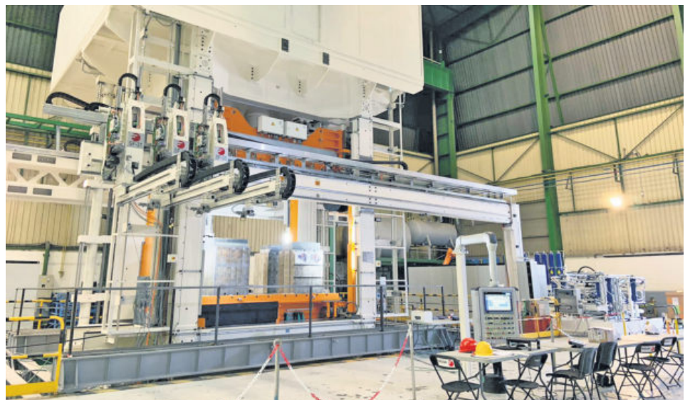
Hot-stamping press under construction at Fagor Arrasate's facilities.
