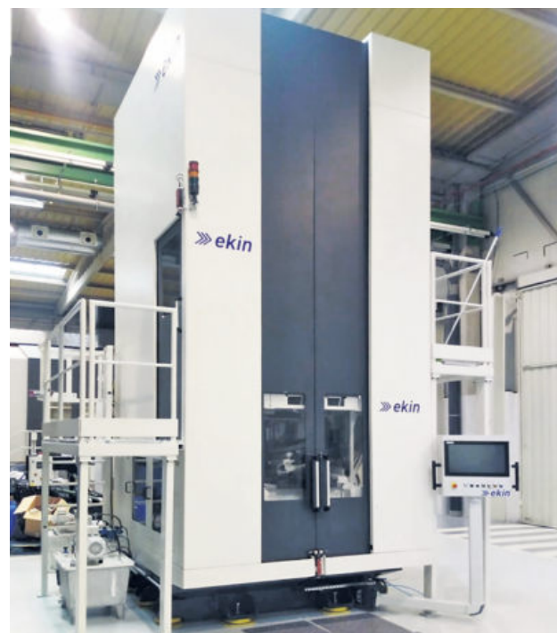
Ekin broaching machine at the Advanced Aeronautics Manufacturing Centre.
