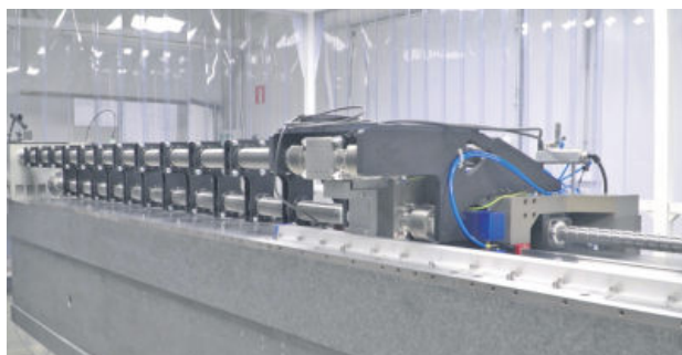
Fagor ultra-precision testbench (10 nm per metre of uncertainty).
