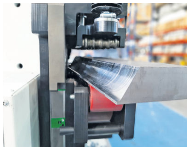
Cevisa also optimises the welding process with its J-shaped chamfer.
