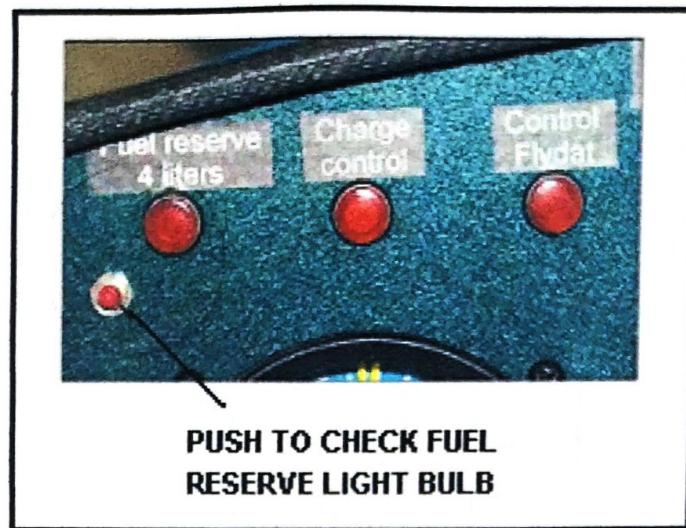
Figure 8 – Control lights and fuel reserve bulb check button
