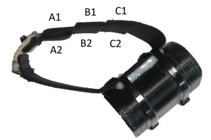
Figure 1. Vectronic Vertex v1.0 collar deployed on white-tailed deer (*Odocoileus virginianus*) fawns at Whitehall Deer Research Facility in Athens, Georgia, USA, during 2018-2019 for testing of experimental designs of Global Positioning System (GPS)-sized expandable radiocollars.
