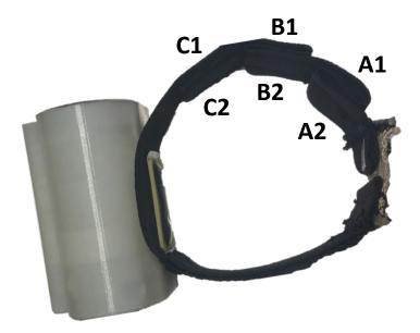
Figure 2. Vectronic Vertex v2.0 collar deployed on white-tailed deer (*Odocoileus virginianus*) fawns at Whitehall Deer Research Facility in Athens, Georgia, USA, during 2019-2020 for testing of experimental designs of Global Positioning System (GPS)-sized expandable radiocollars.
