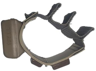
Figure 5. Telonics TGW v2.0 collar deployed on white-tailed deer (*Odocoileus virginianus*) fawns at Whitehall Deer Research Facility in Athens, Georgia, USA, during 2019-2020 for testing of experimental designs of Global Positioning System (GPS)-sized expandable radiocollars.
