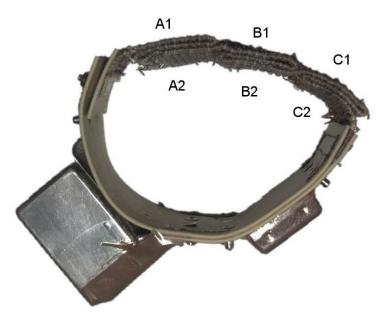
Figure 4. Telonics Recon v1.0 collar deployed on white-tailed deer (*Odocoileus virginianus*) fawns at Whitehall Deer Research Facility in Athens, Georgia, USA, during 2018-2019 for testing of experimental designs of Global Positioning System (GPS)-sized expandable radiocollars.
