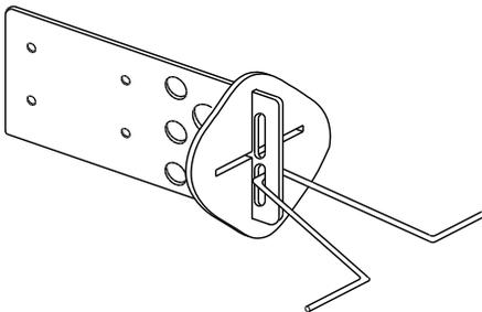
Figure 4 Slotted Stud Tie (Type II) Assembled
