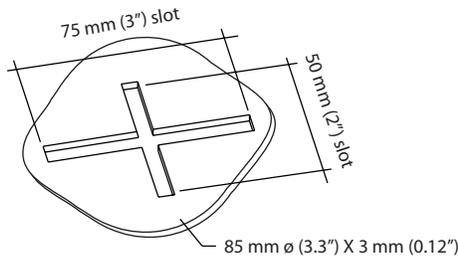
Figure 2 Insulation Support/Retainer
