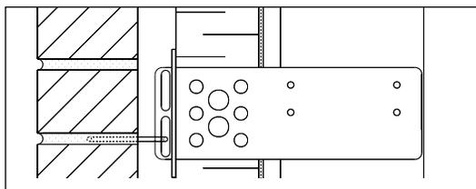
Figure 5 Slotted Stud Tie (Type II) Installed
