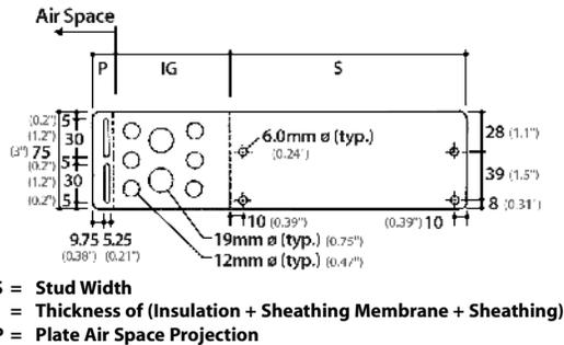
Figure 1 Slotted Stud Plate (Type II)
