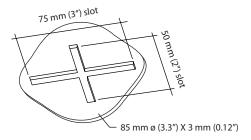
Figure 2 Insulation Support/Retainer
