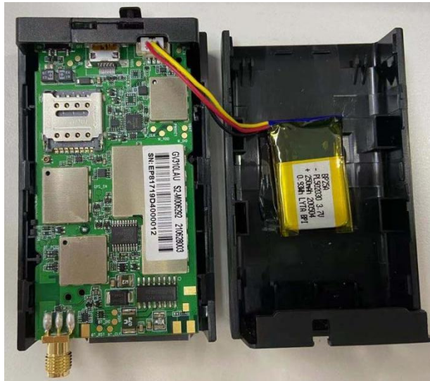
Figure 6. Backup Battery Installation
