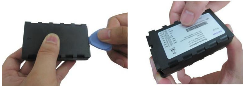
Figure 4. Opening and Closing the Case
