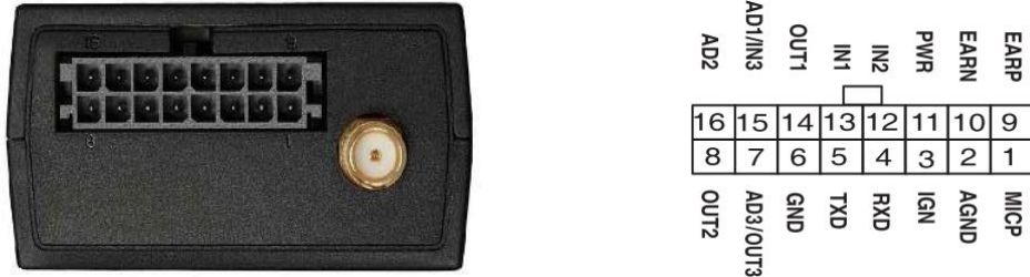
Figure 3. The 16-pin Connector on the GV310LAU
