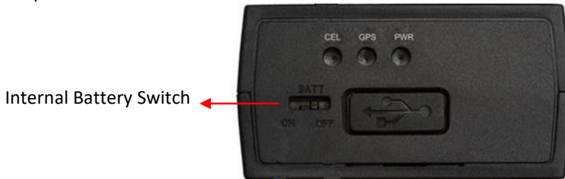
Figure 7. Switch and ON/OFF Position
