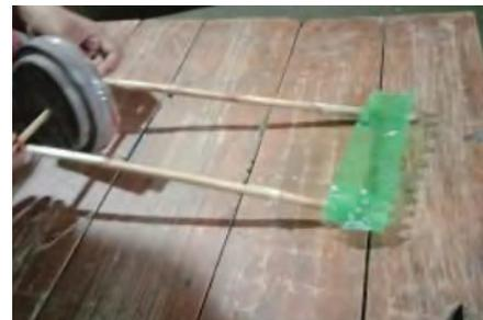
3. Rabia made a model to cut the grass with a fan attached to a rod and the rod attached to the front part of the bicycle. The same fan-like structure is available already, but it runs on electricity, and since there is an erratic supply of electricity in the village, Rabia thought of making a design which can work with bicycle. The grass is fodder, which after cutting can be given to livestock as food.
